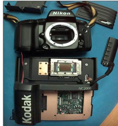
Fig 2.3 Exploded view of a standard digital SLR camera
