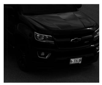
License plate that has been located in the larger vehicle image captured by an LPR camera.
