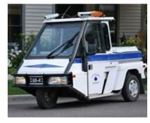
Mobile LPR camera mounted on parking enforcement vehicle.
